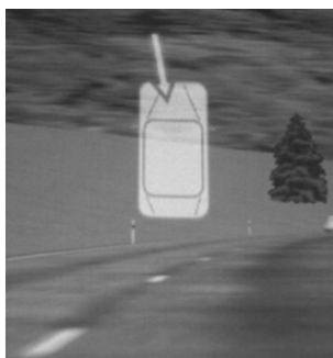
Figure 3. The bird's eye presentation scheme for guidance of attention. A 2D arrow is placed in front of the car with a slight overlap.
