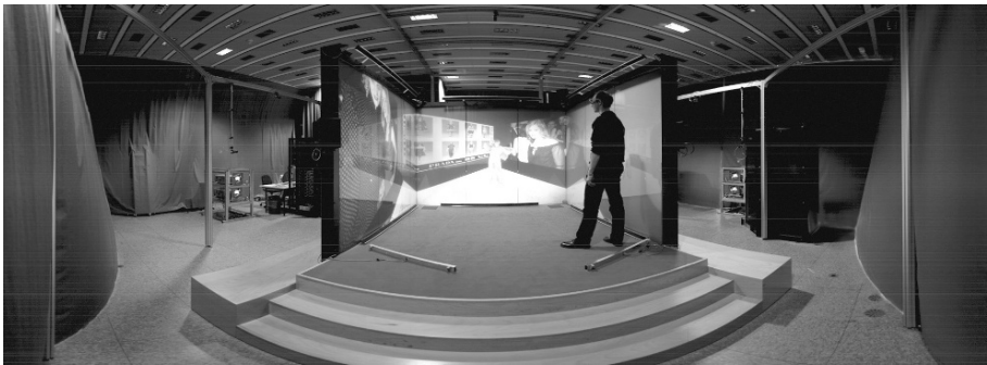
Figure 6. Fisheye view of BlueC. Projectors and cameras are placed outside the glass panels, LED lighting devices on the floor (Copyright ETH Zurich, blue-c.ethz.ch ).
